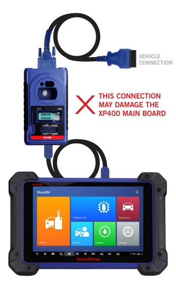
**DO NOT** connect the XP400 to the vehicle directly. The DB26-PIN port is to connect with the Mercedes Benz infrared cable, vehicle key cable, ECU cable, MCU cable, or MC9S12 cable.
